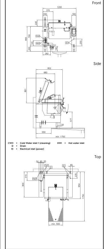
ProThermetic Sprint Electric Tilting Pressure Braising Pan, 90lt Hygienic Profile, Freestanding with CTS The company reserves the right to make modifications to the products without prior notice. All information correct at time of printing.
